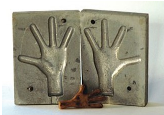
Fig. 8 - Aluminum mould with foam-latex hand. The mould was made by Scheffer and cast in Melbourne. Photo by L. Torre.
